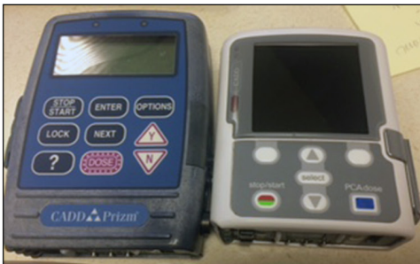
Figure 1: Durable Infusion Pump and Potential Disposable Substitutes
