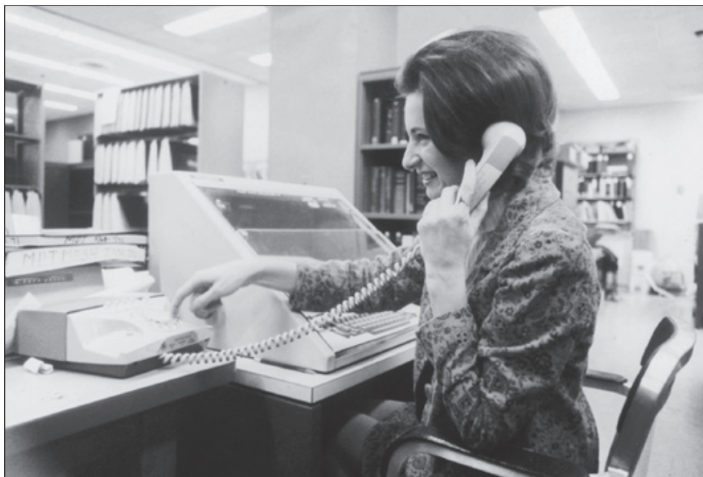
Librarians Gerry Nowak (above) and Yvonne Scott (right) use acoustic couplers (early computer modems) to establish a connection to a mainframe computer, which enabled access to MEDLINE in the mid-1970s.
