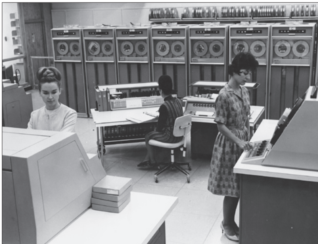
Above, computer operators work with the tape-driven Honeywell 800 mainframe computer, originally acquired by the library in 1963, which ran MEDLARS. The Honeywell 800 ran an assembly language called ARGUS (Automatic Routine Generating and Updating System). Prior to the arrival of the Honeywell computers, General Electric staff trained library staff in using ARGUS.
