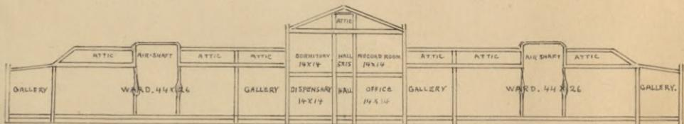
FIG. 20. PLAN OF HOSPITAL - LATERAL SECTION.
