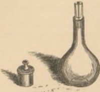
Specific gravity bottle, with tubulated stopper and counterpoise. † 117.
