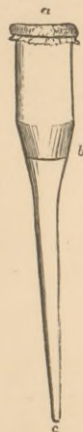
Pipette, serving as the stopper to the bottle. a , vulcanised india-rubber, by pressing which fluid may be expelled from the tube. b , ground to fit the neck of the bottle. c , the orifice. § 139.
