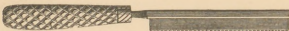
Fine saw, for cutting thin sections of bone and teeth, which are afterwards to be ground thinner on the hone and polished as described in § 95.
