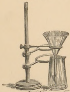
Retort stand, funnel, and glass, arranged for filtering § 108.
