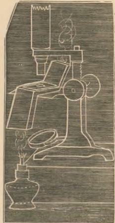
Apparatus for examining objects while exposed to heat. The chimney through which the heated air passes is made of thin copper without being soldered. Both sides are perforated, the lower one being filled up with a piece of glass, while over the upper opening the slide with the object is placed. † 122.
