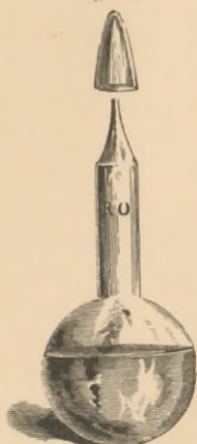
Bulb, with capillary orifice, for testing small quantities of matter. § 138.
