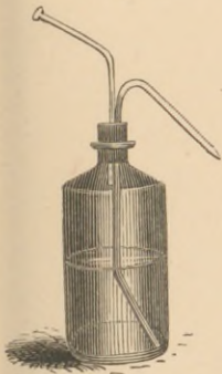
Wash bottle, for washing preparations. A stream of water is projected from the orifice of the pipe, when air is blown into the upper tube. † 107.
