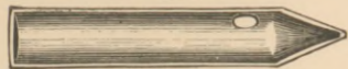
Glass tube for containing solutions for examination under the spectrum microscope. Half the real size. § 173.
