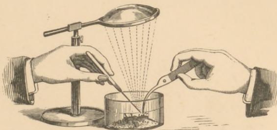
Arrangement for dissecting objects under water. The bull's-eye condenser is much larger than those usually employed. § 95.
