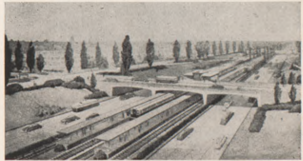
Typical Cross-Section Showing Superhighway and Four-Track Subway
