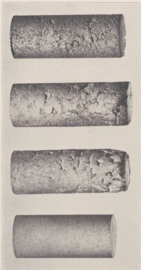
Fig. 87.—Results of correctly and incorrectly amalgamating same high A grade dental alloy. All cylinders packed under 25 kg. per cir. cm. in same mould. Wrong manipulation yields amalgam that is difficult to condense and to adapt to cavity walls. Cracks and folds weaken. Slow diffusion of mercury trapped in voids causes large and long-continued volume changes. \times 4 . Bottom surfaces of same specimens \times 25 are shown in Figs. 83, 84, 85, and 86.
