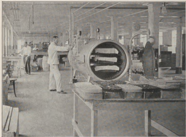
Section of the sterilization room of the Johnson & Johnson Laboratories. The high pressure steam sterilizer, shown in the foreground, has a normal working capacity of 10,000 tubes.
