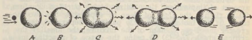
Fig. 34 Fission of Uranium Caused by Neutron Adsorption.
