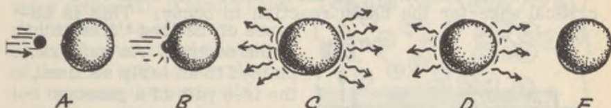
Fig. 35 Neutron Absorption by Uranium Without Fission Production.
