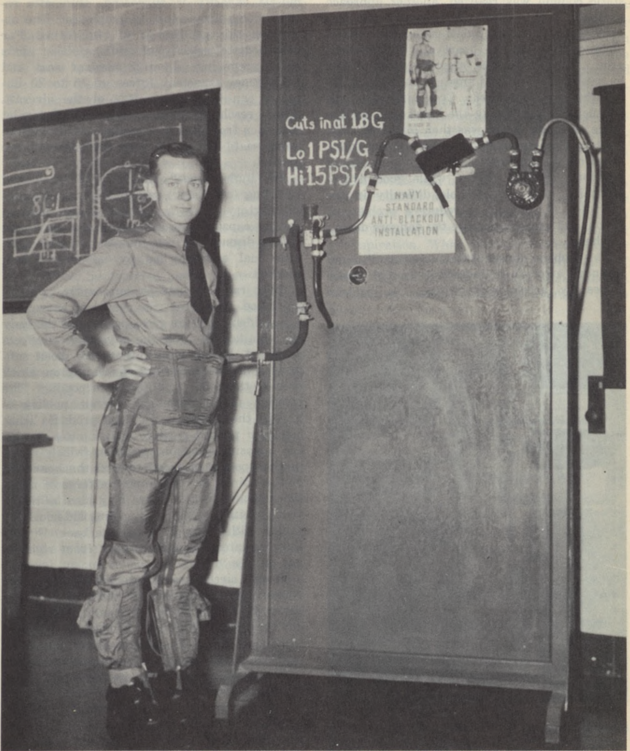
Figure 3-4.—The Standard U. S. Navy Z-3 anti-blackout suit. This is a cut down model of the Z-2 suit. It may be worn over the underwear and under or over conventional uniforms. It incorporates the air bladder systems of the Z-2 in a form which can be worn with many other clothing arrangements. As pictured it is partly inflated.
