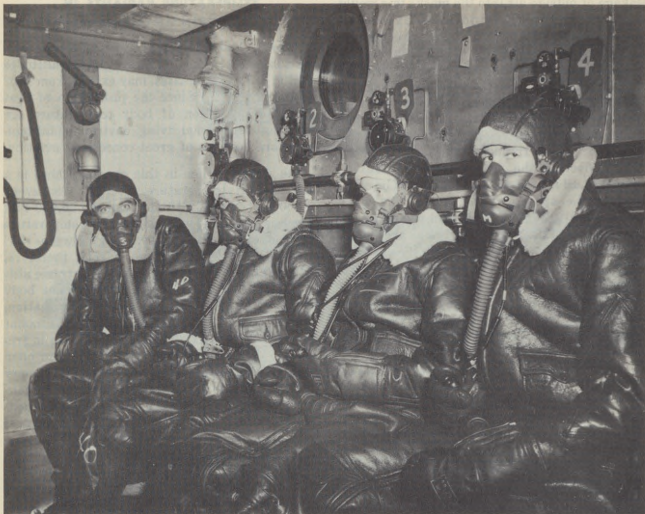
Figure 2-12. —Subjects receiving instruction in the handling of oxygen equipment during a chill run in a low pressure chamber. Navy standard aviator's cold weather shearling clothing is being worn.
