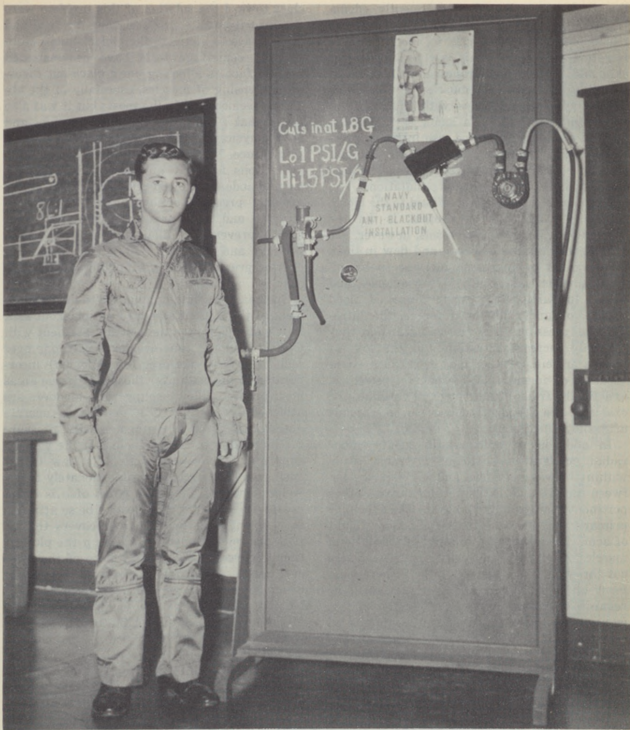
Figure 3-3.—The Standard U. S. Navy Z-2 anti-blackout suit partly inflated (note abdomen). Note also the air source is attached by means of a quick disconnect on the left. Also pictured is a standard G-valve and oil filter to demonstrate, statically, the method by which the suit fills under simulated G. This suit can be worn in place of the conventional coverall and is light weight and porous for skin ventilation. It may be worn under cold weather gear without discomfort or impairment.
