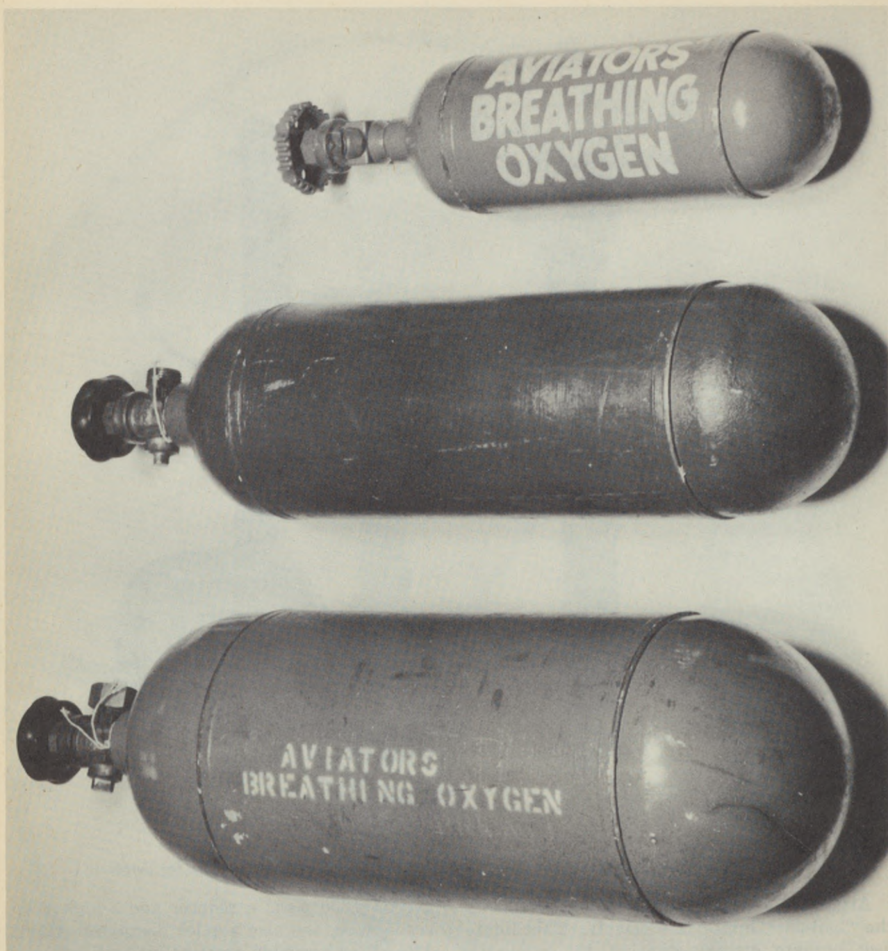
Figure 2-11.—Navy high pressure oxygen bottles for use in aircraft oxygen systems. Bottles are 504 cu. inch, 205 cu. inch and 96 cu. inch capacity.
