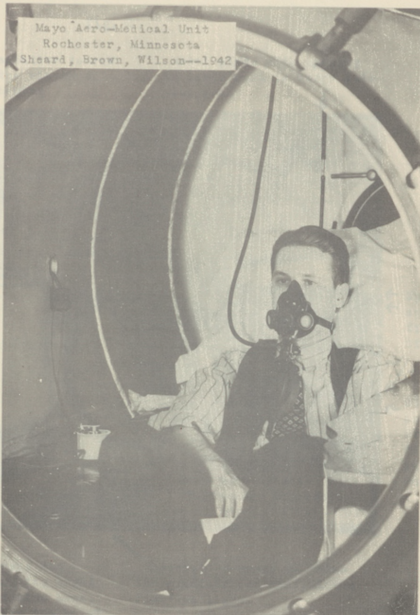
Subject wearing BLB Aviation mask sitting in position in the low pressure chamber.
