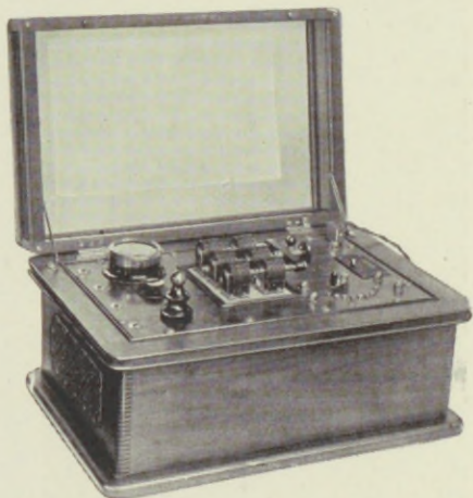
FIG. 7. Improved portable diathermy apparatus with multiple spark gap and three variations of diathermy current.
