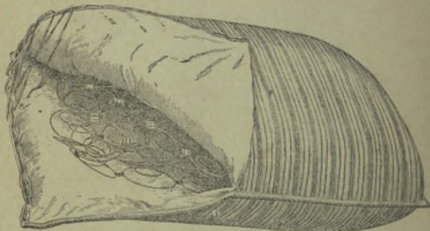
Pillow open and cut to show construction
