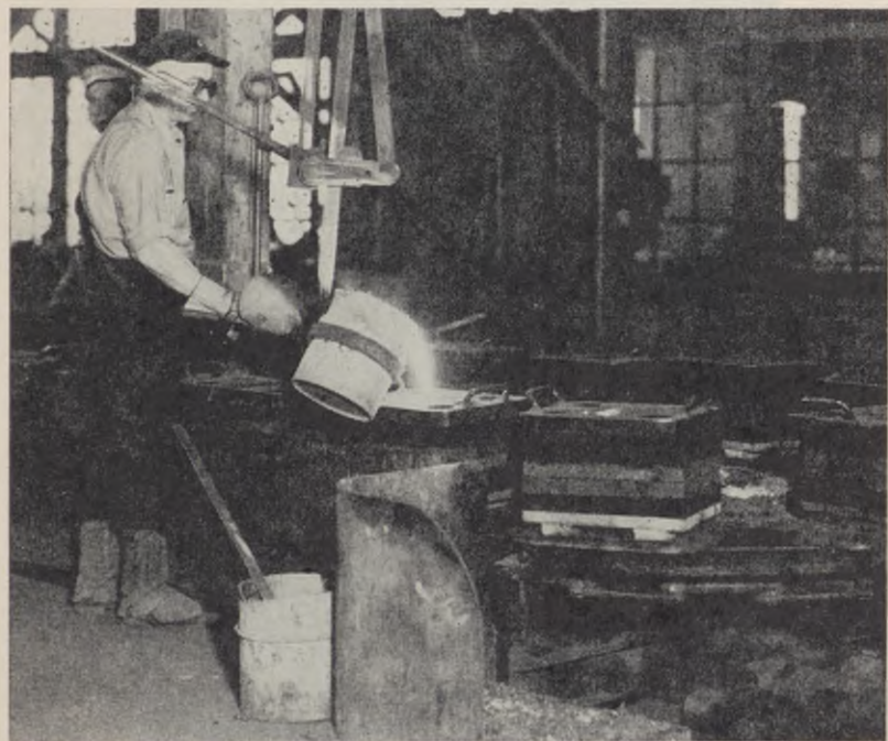
Pouring Station of Mold Conveyor
