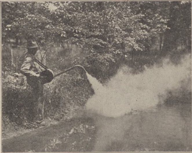
Fig. 58. Hand duster blower for Paris green. (From Dunham's Military Preventive Medicine , 3rd Edition).
