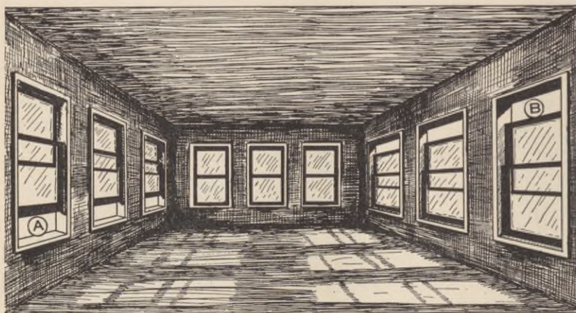
Fig. 41. Natural ventilation with open windows. (From Dunham's Military Preventive Medicine, 3rd Edition).
