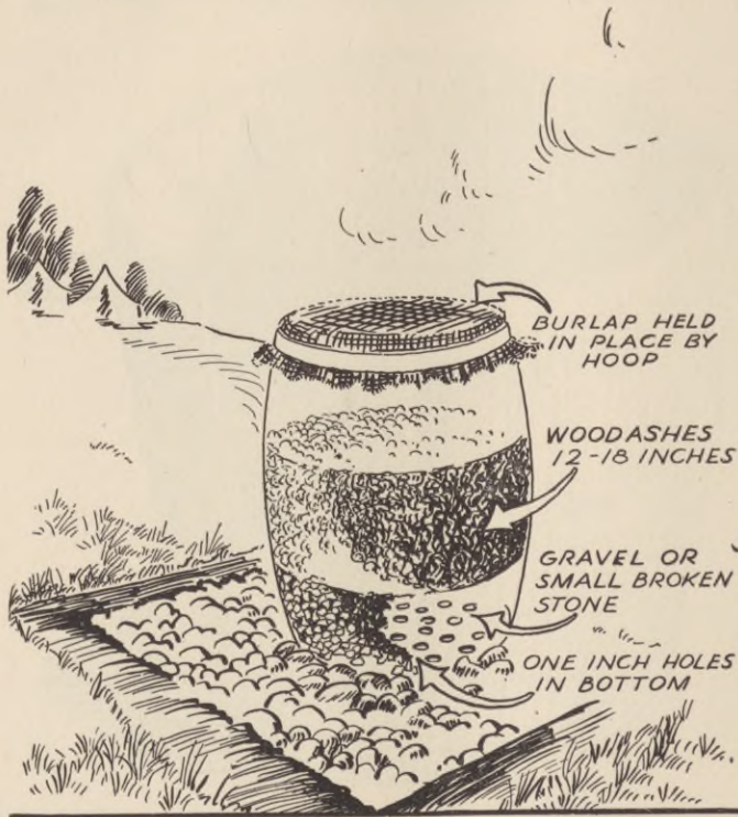
Fig. 28. Ash barrel grease trap.
