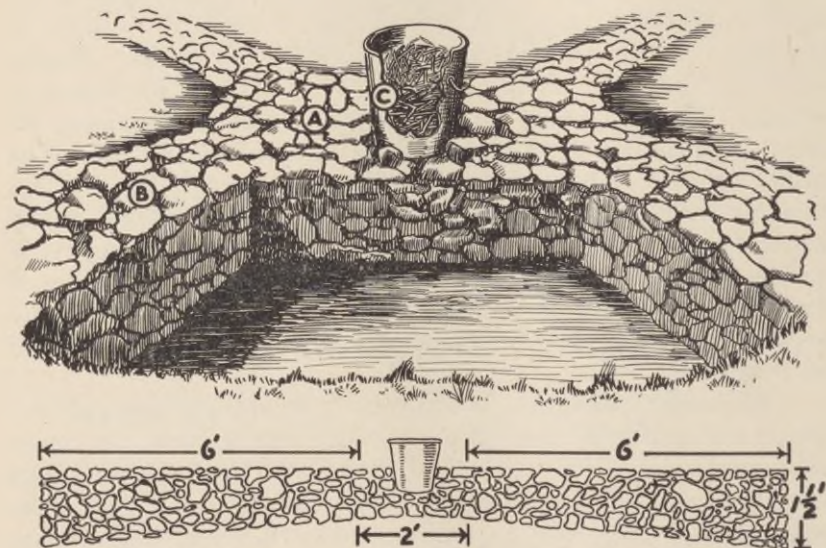
Fig. 29. Soakage trench. A—Central square area; B—Radiating lateral trenches; C—Pail grease trap. (From Dunham's Military Preventive Medicine, 3rd Edition).
