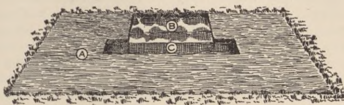
Fig. 22. Method of flyproofing latrine. A—Layer of earth replaced and tamped down over burlap. B—Oiled burlap exposed before replacement of earth. C—Opening of pit. (From Dunham's Military Preventive Medicine, 3rd Edition).
