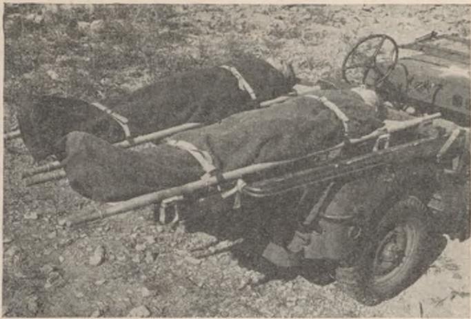
FIGURE 164.—Two litters loaded onto permanent frame.
