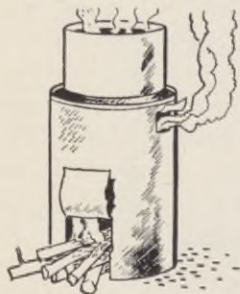
A tin-can stove. A large can makes a good stove, cut stoke-hole and flue
