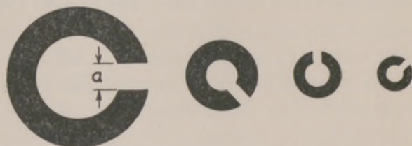
Fig. 36. The international test-object for visual acuity. The dimension of the opening a determines the visual angle when distance from the eye is taken into account. The subject not only must see the discontinuity of the ring but must state in what position it is. Several sizes and positions are reproduced herewith so that the reader may compare them at a distance at which the smallest is not seen as a split ring.
