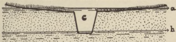
Fig. 21. Lowering of ground water by means of a ditch; a, ground water level before digging ditch; b, ground water level after digging ditch; c, drainage ditch.
