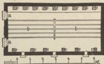
Fig. 254. Inner arrangement of a chicken house. a , Doors; b , roosts; c , nests.
