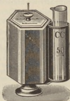
Fig. 30. Colorimeter for determination of ammonia.
