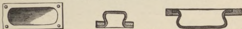
Fig. 202. Correct shape of iron manger. a, Manger from above; b, cross section; c, longitudinal section.
