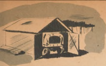
OPEN GARAGE DOORS WHEN RUNNING ENGINE.
