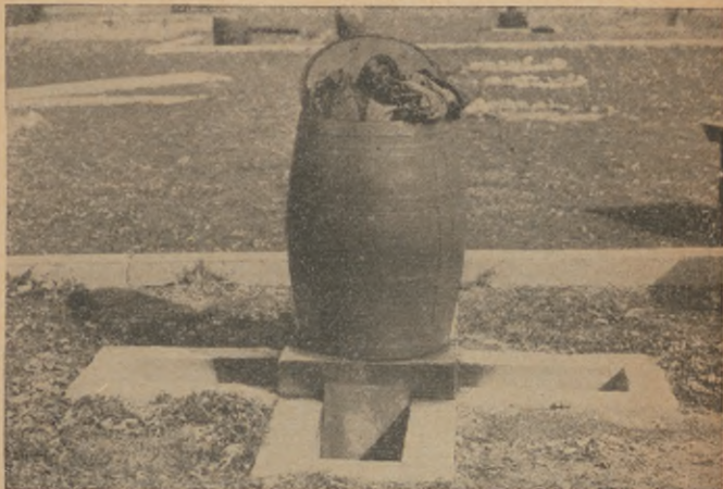
FIGURE 53.—Disinfestor, Serbian barrel type.
