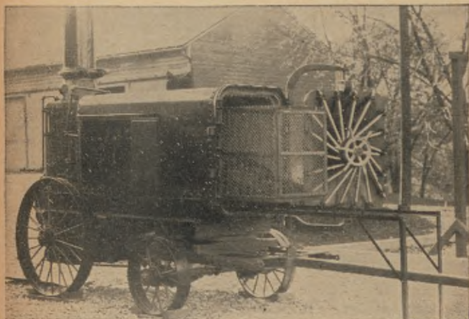
FIGURE 52.—Portable pressure disinfestor.
