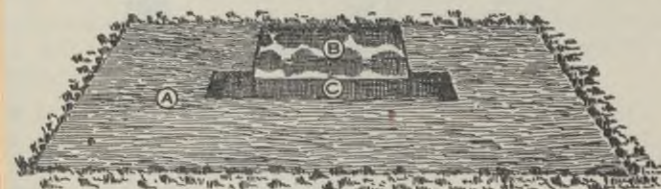
FIGURE 9.—Method of flyproofing latrine pit with oiled burlap. A—Layer of earth replaced and tamped down over oil-soaked burlap. B—Oiled burlap exposed before replacement of earth. C—Opening of pit.
