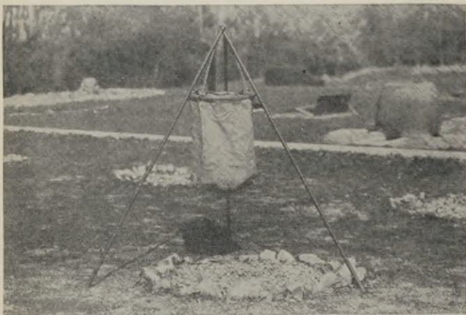
FIGURE 6.—Water-sterilizing bag suspended from tripod.
