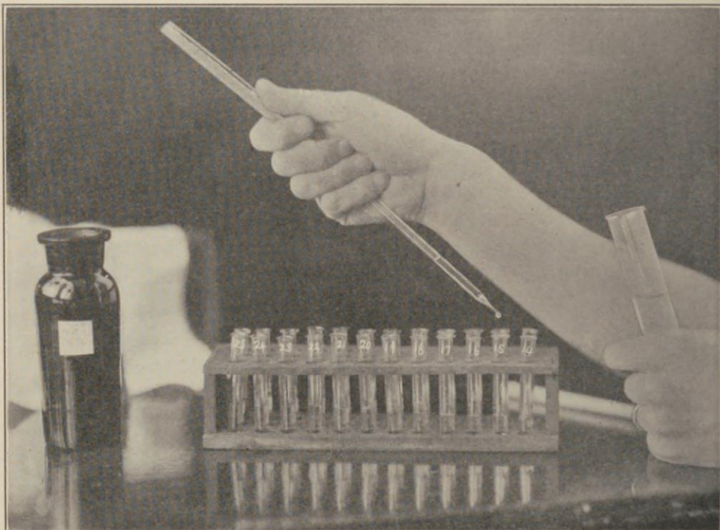
Fig. 39.—Dilutions are made of 0.5 per cent sodium chloride solution by adding distilled water by the drop method so that each tube contains twenty-five drops of hypotonic solution. (After Giffin and Sanford.)
