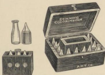
Fig. 24.—Dunning colorimeter used in phenolsulphonephthalein test of kidney function.
