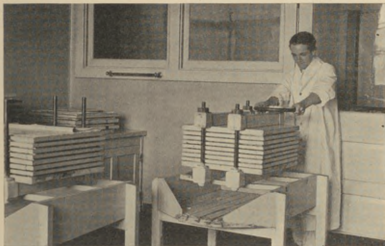
FIG. 68—Drying the precipitate containing the antitoxic globulins, by pressing out the water. The precipitate is placed between many thicknesses of absorbent filter paper; several lots of such precipitate (separated by boards) may be pressed nearly dry in the same press as shown in the accompanying illustration. H. K. Mulford, Co.
