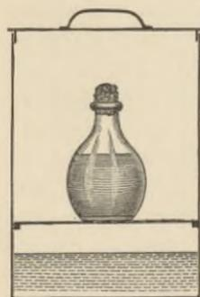
cover should be tight so as to hold in the steam and prevent the ingress of air. For use, two or three inches of water should be placed in the bottom and brought to a fast boil, when the flasks should be set as near the centre of the diaphragm as possible, the cover replaced, and the whole allowed to steam for fifteen minutes. The flasks should then be taken out and stood in the cold; of course, to be brought up to the body temperature before feeding.
