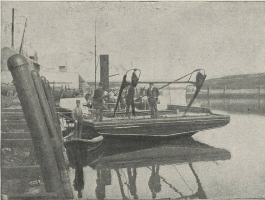
FIG. 1. HOLLAND. A NETHERLANDS STEAM OYSTER DREDGE, A SIDE-WHEELER EXTREMELY BROAD OF BEAM (BELONGING TO MR. OCHTMANN, BERGEN-OP-ZOOM).
