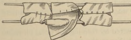
Fig. 15.—Litter constructed of two poles thrust through the sleeves of three blouses.
