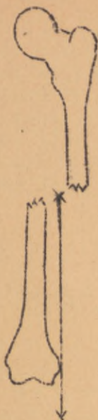
Illustration 69. Elimination of the lateral component to the longitudinal traction force by shifting the point of attack of that force to the fracture cleft. At any angle of the distal fragment that component force will be equal to zero.
