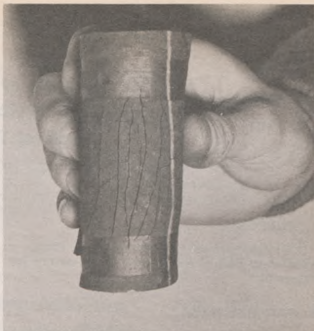
Outer covering cracked on aromatic resistant oil hose
