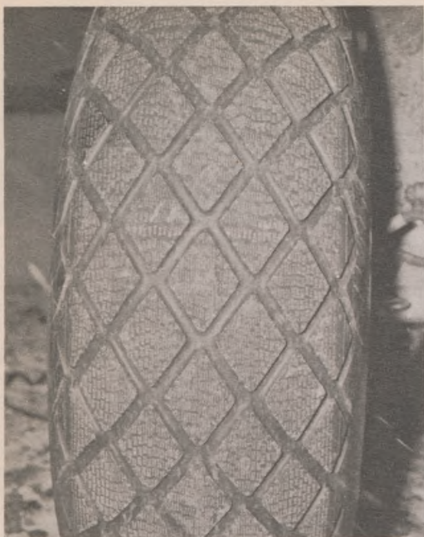
Ice grip tire with steel spring inserts
