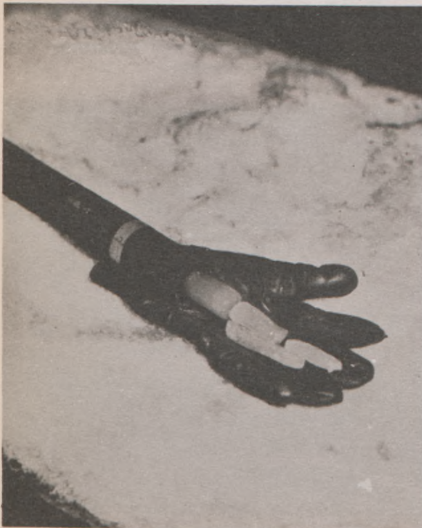
Ice found in fuel inlet line
