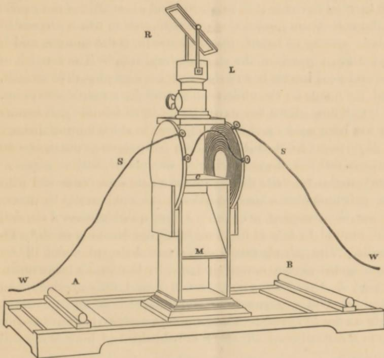
not only approach to and recede from the lantern, and thus alter their distances from the galvanometer-needle, but they can also rotate around their centers on vertical axes. The like poles of the magnets and of the needle point in the same direction; and by sliding the magnets to or from the lantern-needle we render the latter more or less astatic. Also, in case the needle should not hold to the meridian as you approach the magnets,
