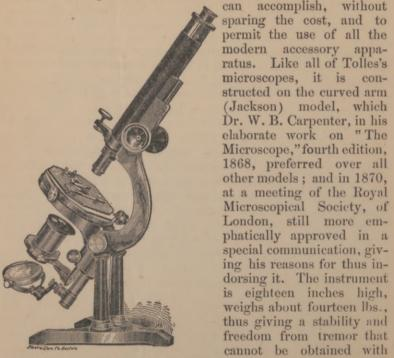
stands of little weight. It is of simple construction, with fewer screws and pieces than any other first-class micro-
