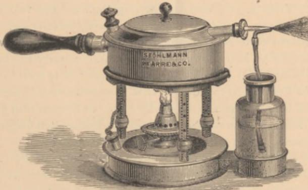
its diminished cost some of the improvements of Mr. Lister's lamp have been sacrificed. It is, however, essentially the same. Its hollow wick, readily raised or lowered, affords a great and controllable heat. The spray-tube is in this apparatus fixed, an objection which in the majority of cases is of no moment. It will supply spray for over two hours. It therefore requires only that the boiler—containing twenty-two ounces—should be, as well as the lamp, full at the beginning
