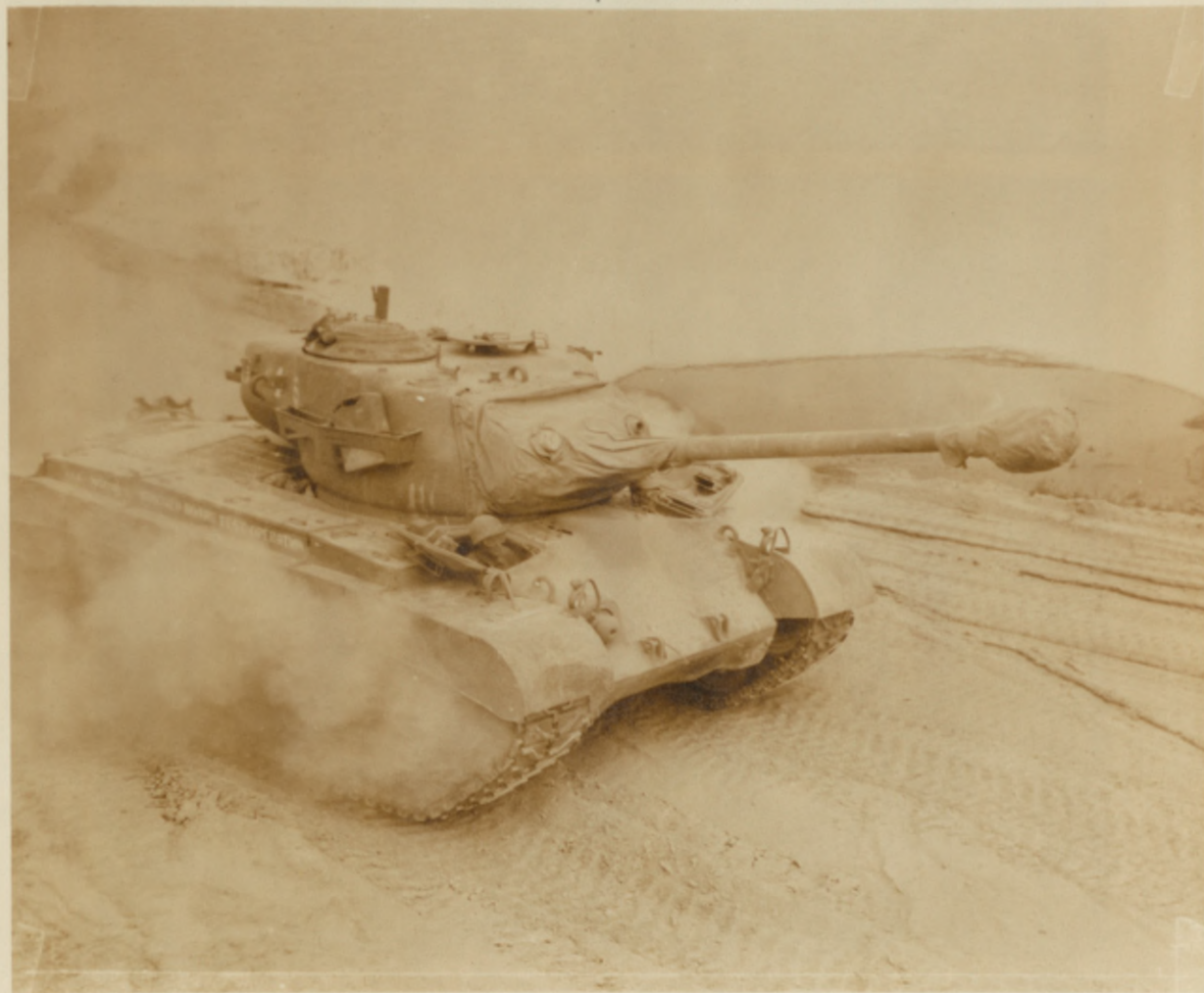
Dust Pattern for Heavy Tank, M26 with Fenders and Sand Shields ARMORED MEDICAL RESEARCH LABORATORY FORT KNOX, KY. July, 1945
