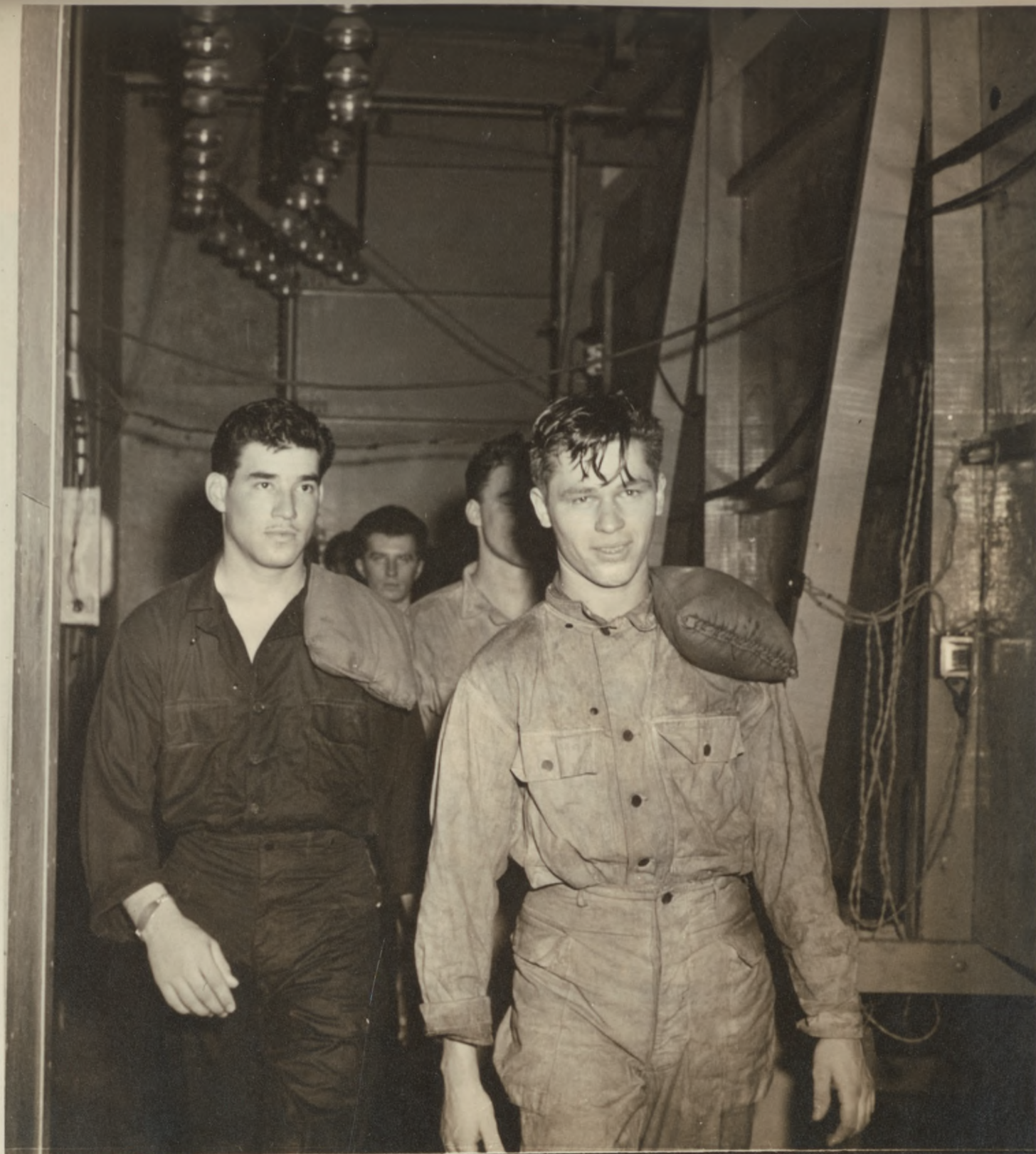
HBT Appearance of herringbone twill garment during twelfth wearing compared with that of flameproof twill during fifth wearing. ARMORED MEDICAL RESEARCH LABORATORY
