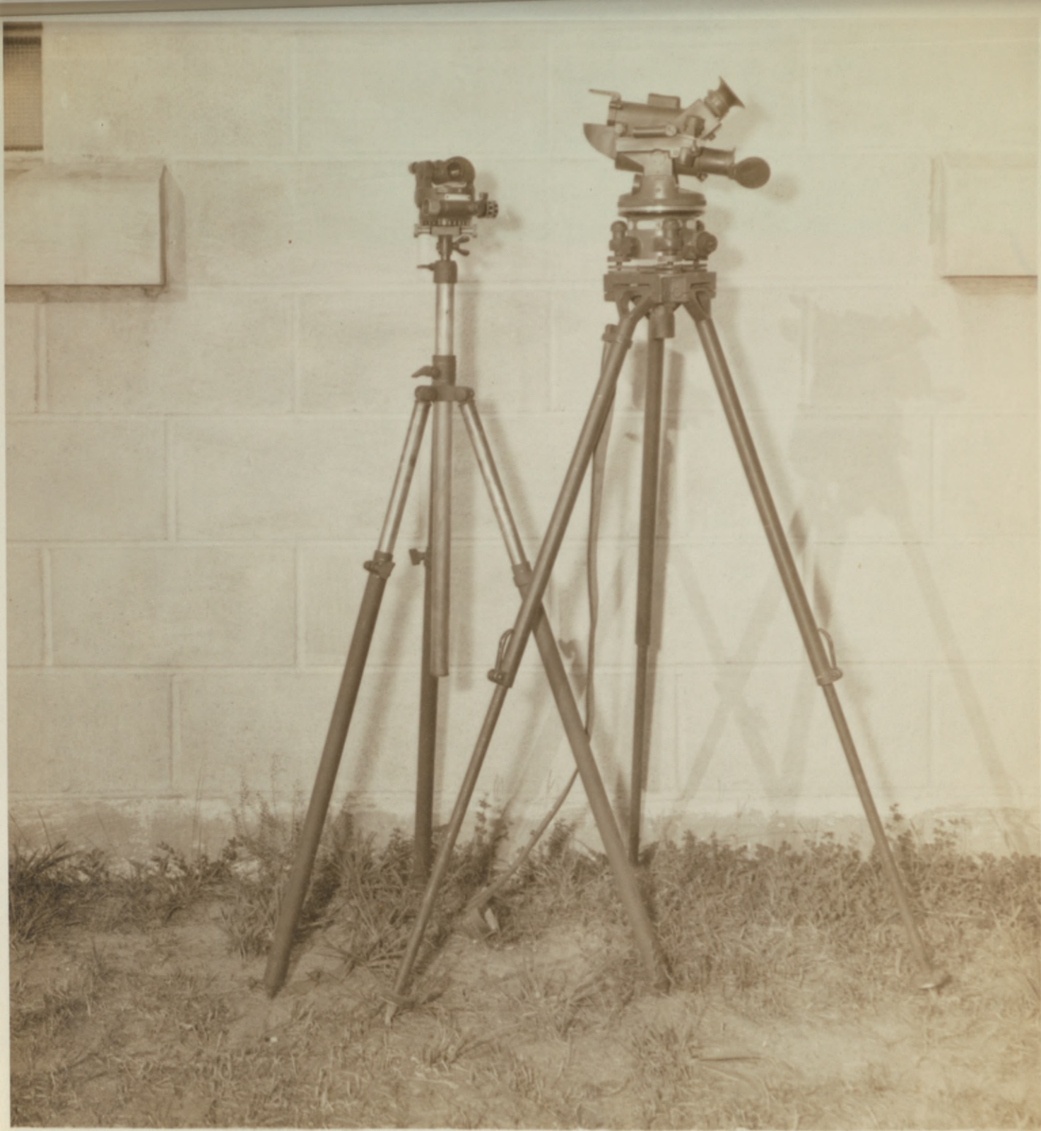
AIMING CIRCLES AMERICAN M1 (LEFT) AND GERMAN (RIGHT) ARMORED MEDICAL RESEARCH LABORATORY FORT KNOX, KY.
