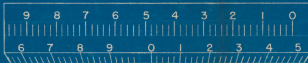
Micrometer Scale (Unrolled view) Note Gap from 9.8 to 0
