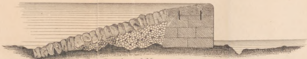
Section of Masonry Dam
