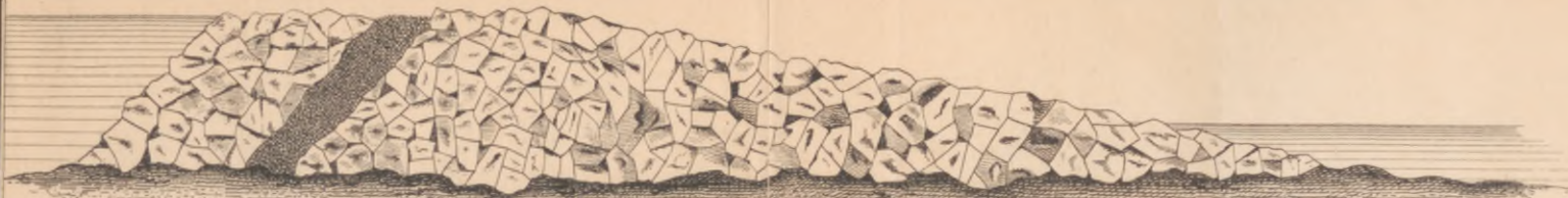
Section of Embankment of Rubble Stone
