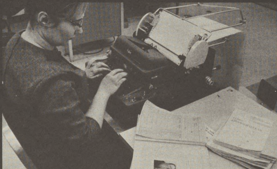
8. PUNCH PAPER TAPE DATA-INPUT TYPEWRITER - MEDLARS
