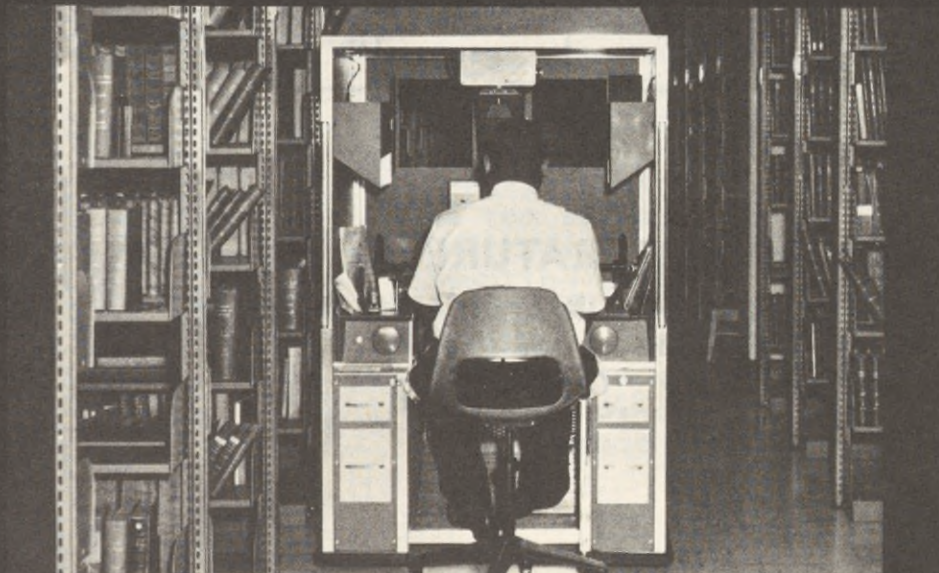
7. MOVABLE CAMERA WITHIN STACK - PHOTOGRAPHY FROM PAGE TO MICROFILM
