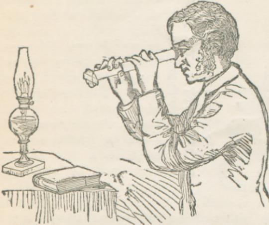
For clinical and field or sea-side use, is a simple tube 6 inches long, with a one-quarter inch Objective and B Eye-Piece, — fine and coarse adjustments for focus, — a Stage with spring-clips to hold the object, which can be removed when not in use, and the Objective covered
