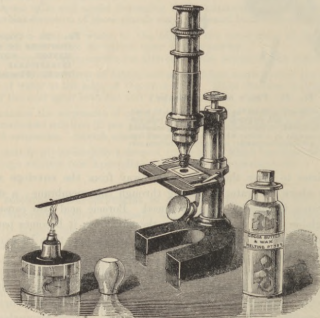
FIG. 27.—SIMPLE WARMING APPARATUS, COMPLETE, SHOWN IN OPERATION.
