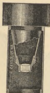
FIG. 149. Zeiss' Apochromatic, Projection Objective of 70 mm. equivalent focus, for photo-micrography. (Zeiss' Catalog. No. 30). This, and another of 35 mm. focus, are designed for making pictures of moderate magnification. Usually rather large objects are photographed with them. The object may be illuminated in the ordinary way. They are used without an ocular, like a photographic objective. The one of 35 mm. is screwed into the tube of the microscope like an ordinary objective, but the one of 70 mm. here shown, is, by means of a conical adapter, screwed into the ocular end of the tube.
