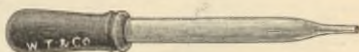
FIG. 133. Pipette for adding liquids dropwise and for washing preparations. (Whitall, Tatum & Co.)
