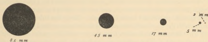
FIG. 37. Figures showing approximately the actual size of the field with objectives of 85 mm., 45 mm., 17 mm., 5 mm., and 2 mm., equivalent focus, and ocular of 37\frac{1}{2} mm., equivalent focus in each case. This figure shows graphically what is also very clearly indicated in the table (§ 47).
