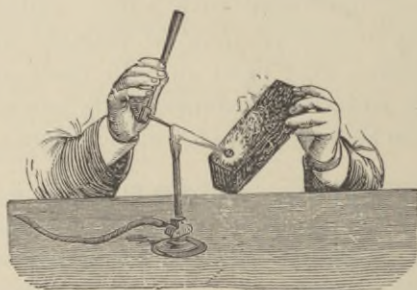
Heating on charcoal by means of blowpipe.
