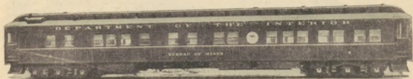
New all-steel mine rescue car of the Bureau of Mines.
