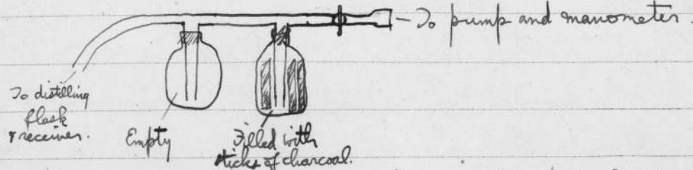
After exhausting most of air, immerse the two bulbs in Dewar flasks cont. liquid air. Charcoal takes up all air left.
