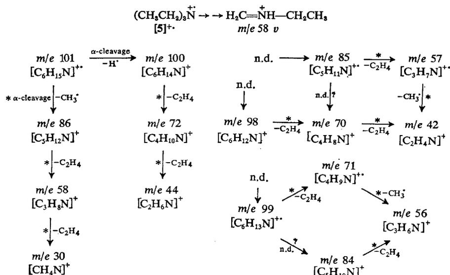
SCHEME 2. Metastable map indicating pathways of fragmentation of  $[(\text{CH}_3\text{CH}_2)_3\text{N}]^+$  (**5**).†
