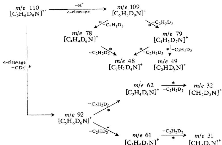
SCHEME 3. Metastable map indicating pathways of fragmentation of  $[(\text{CD}_3\text{CH}_2)_3\text{N}]^+$  (**6**).
