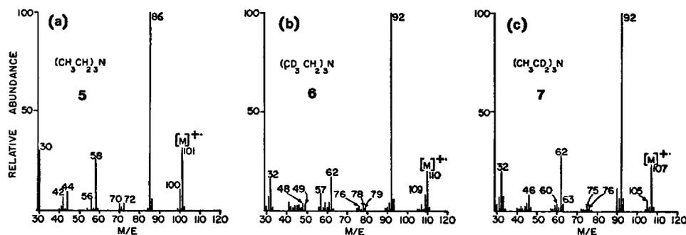
FIG. 1. (a) Low resolution mass spectrum of triethylamine (5); (b) low resolution mass spectrum of 2,2,2,2',2',2'',2'',2''-nonadeuteriotriethylamine (6); (c) low resolution mass spectrum of 1,1,1',1'',1''-hexadeuteriotriethylamine (7).
