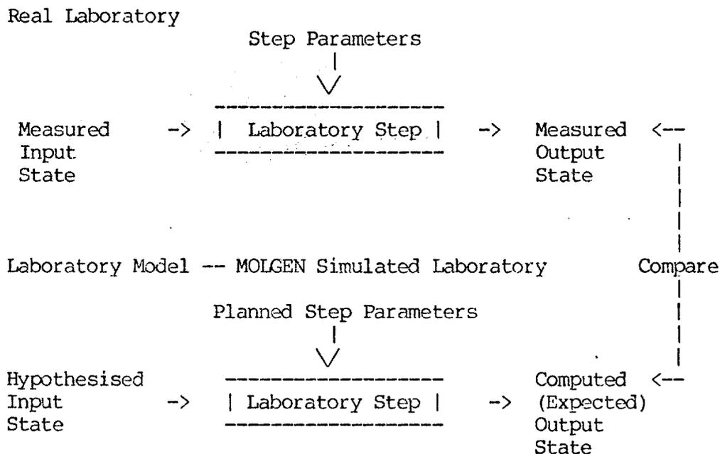
In this diagram, we assume that a complete plan for a laboratory experiment has been developed. In this diagram, we will focus on a single step in the experiment. The upper part of the diagram corresponds to the step as carried out in the laboratory -- illustrating that a laboratory sample undergoes processing in a laboratory step resulting in a changed sample. Measurements are made on both the input and output samples. (4)
