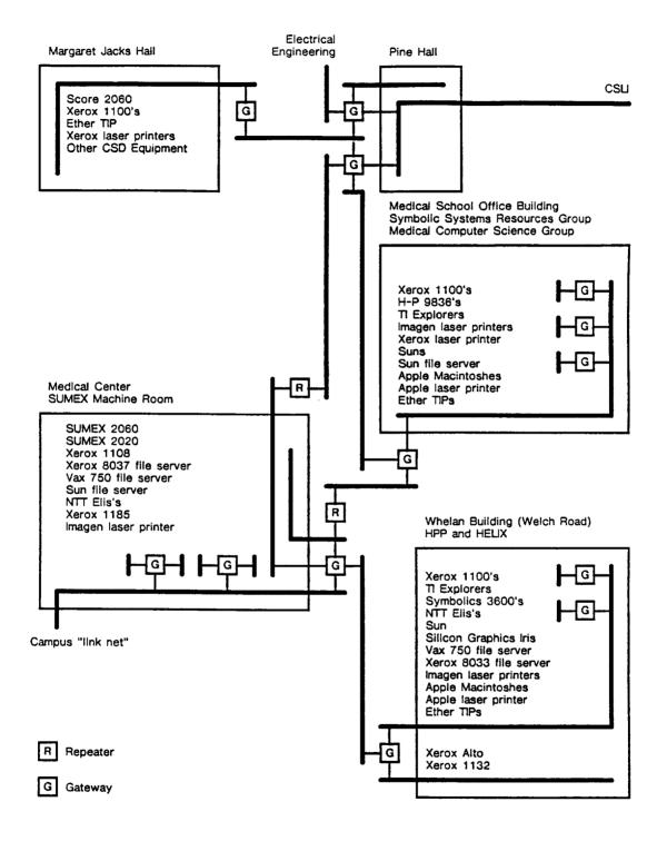
Figure 9: SUMEX-AIM Ethernet Configuration
