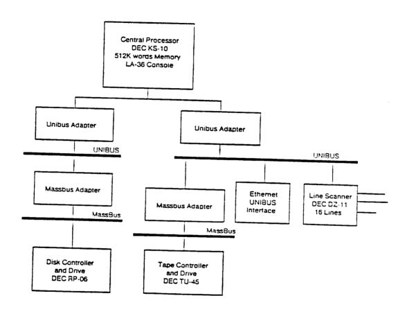
Figure 2: SUMEX-AIM DEC 2020 Configuration
