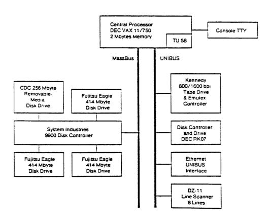
Figure 4: SUMEX-AIM File Server Configuration
