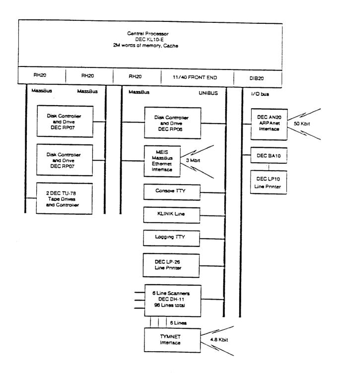
Figure 1: SUMEX-AIM DEC 2060 Configuration
