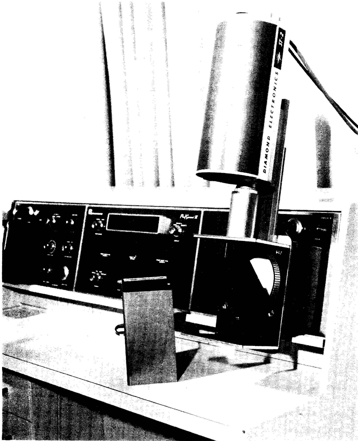
Figure 3. Television camera mounted above scintillation camera display tube.
