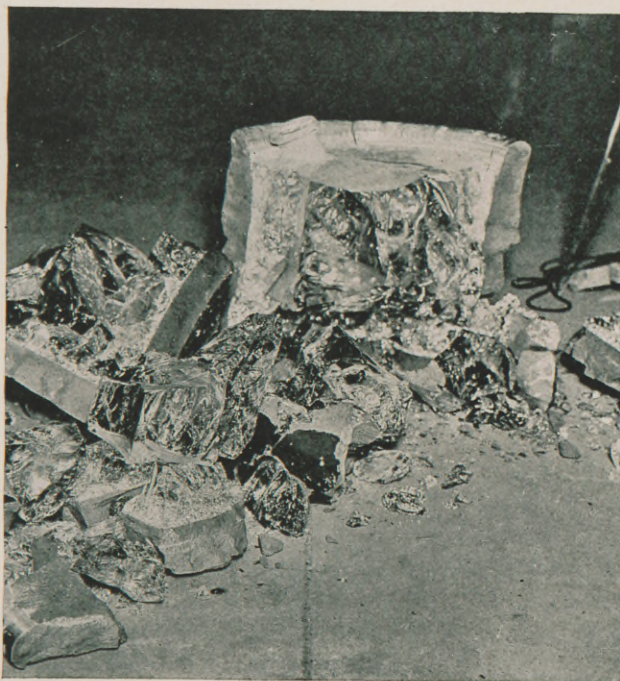
Pot of Optical Glass in Process of Being Broken Up
