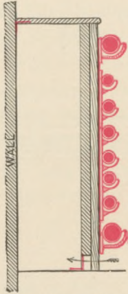
Fig. 74. — Section Through Ventilating Duct.
