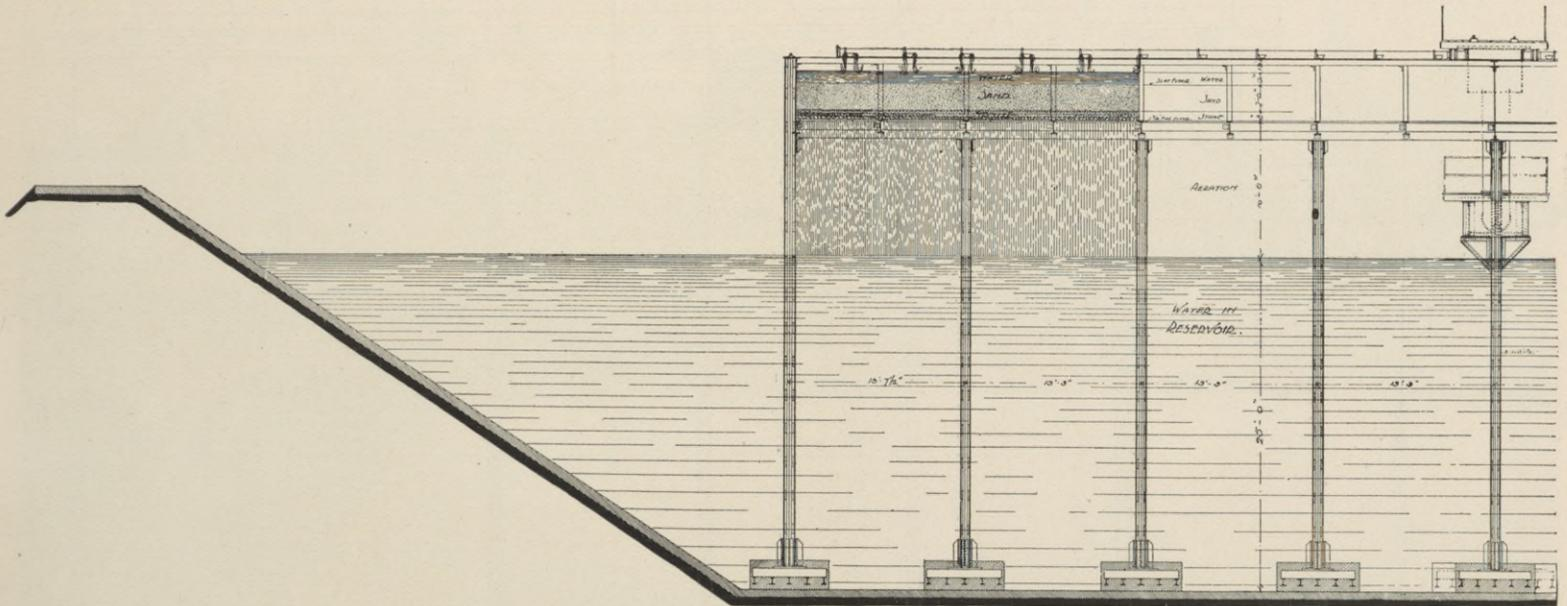
TRANSVERSE SECTION THROUGH ELEVATED FILTER BEDS LOCATED IN AND OVER RESERVOIRS.
