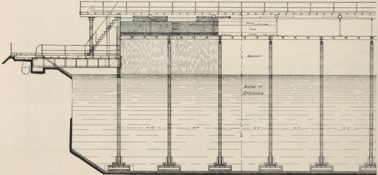
LONGITUDINAL SECTION THROUGH ELEVATED FILTER BEDS LOCATED IN AND OVER RESERVOIRS.
