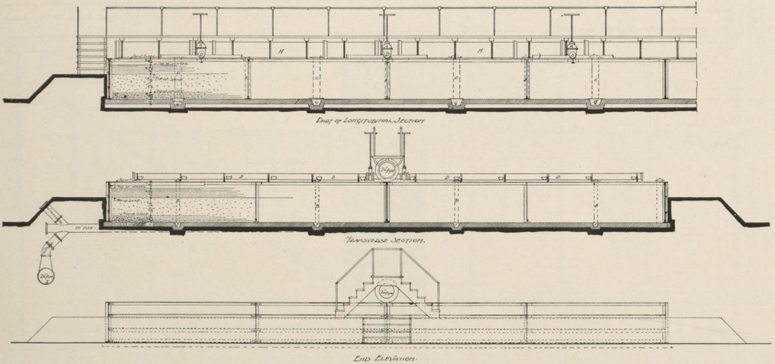
ELEVATION AND SECTIONS OF FILTER BEDS ADJACENT TO RESERVOIRS.
